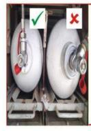
CHECK OXYGEN CYLINDER FOR CORRECT POSITION
