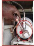
OPEN OXYGEN CYLINDER VALVE TO REQUIRED LEVEL
