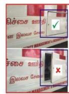
CHECK OXYGEN CYLINDER DOOR FOR PROPER LOCKING
